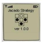
You can click any key to display the next screen, the "Main Screen". If you do not click a key, automatically after 2-3 seconds the "Main Screen" will be displayed.
